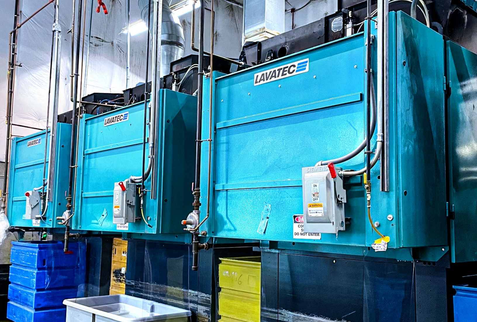
In addition to the tunnel washer and extractor press, Metro Laundry Service utilizes LAVATEC gas dryers as part of its operation.
