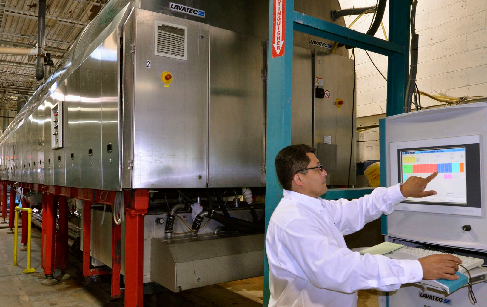
JVK's Operations Manager Jesus Pereira monitors performance data of their 200-pound 16-compartment Lavatec tunnel in the Amityville, New York plant.
